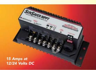
Morningstar's **SunSaver MPPT** solar controller with TrakStar Technology™ is an advanced maximum power point tracking (MPPT) battery charger for off-grid photovoltaic (PV) systems. The controller features a smart tracking algorithm that maximizes the energy harvest from the PV and also provides load control to prevent over discharge of the battery.
