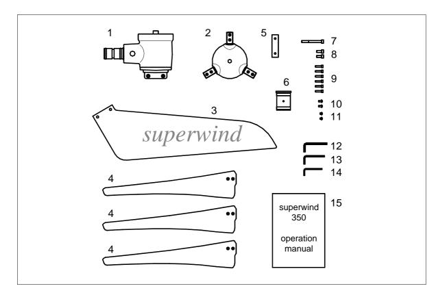
NOTE: For aerodynamic reasons the rotor blades' trailing edges are very thin and sharp. When unpacking the parts you should be careful, in order to avoid injuries.
